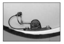
1. Remove pin from inside trailer foot well.
