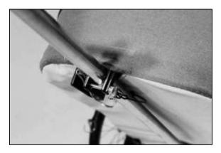
6. Secure tow bar in front foot with tab lock pin. Lock pin in place with wire.
