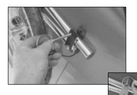
3. Insert locking pin. Lock pin in place with ring by flipping ring over the black plastic receiver.
